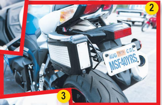
**Photo 2** The data collected by all of the bike's sensors gets recorded to a hard disk inside this sturdy case. If it fills up prior to the completion of the year's testing, a new disk can be swapped in. Note the rear view camera on the bottom.
