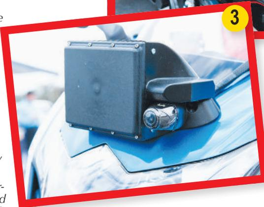
**Photo 3** The forward facing unit carries a camera and a sophisticated radar unit that can simultaneously track multiple objects in the motorcycle's path of travel.
